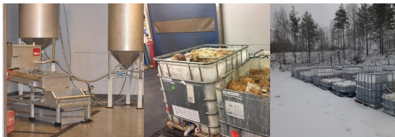
Figure 3. Wood floor industry AB Gustaf Kährs. (a) Part of the demo plant constructed to treat the wastewaters generated indoors; (b) sludge/solid waste removed from the wastewater streams with the new treatment; (c) demo plant for stormwater treatment.
