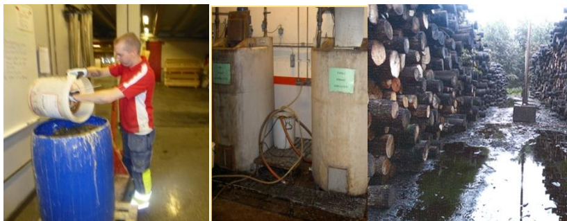
Figure 2. (a),(b) Earlier handling of cleaning/washing wastewater streams at AB Gustaf Kährs and (c) polluted water runoff (leachate) after irrigation of logs, rainfall or snowmelt.
